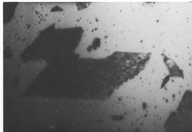
Figure 5 Typical crystals of dodecamethylenediammonium sebacate ( \times 100 )
